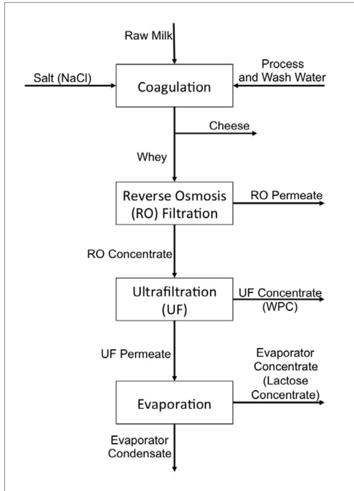
Figure 1. Block diagram for process line.
