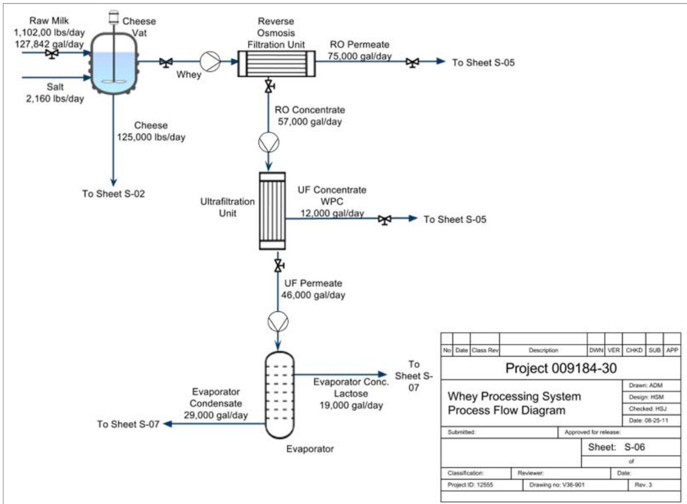
Figure 2. Theoretical flow rates for whey processing line.
